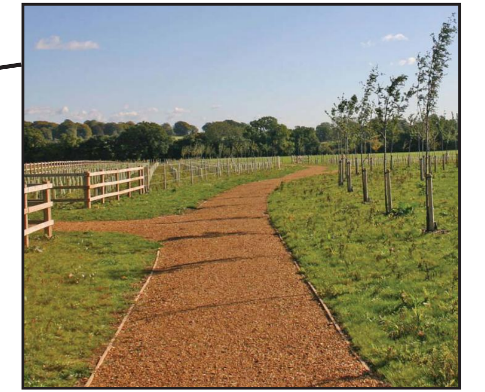
Recreational footpaths surfaced in hoggin with timber edgings; 2-2.5m wide, provides suitable routes around the park and encourages users not to stray into ecologically sensitive areas. NB:- Restricted vehicle access will be permitted for maintenance.
